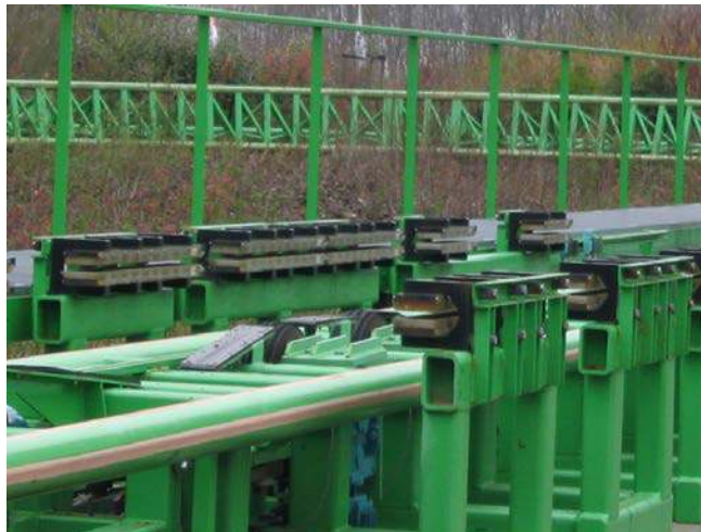
Figure 23.19 The rows of rare earth magnets (protruding horizontally) are used for magnetic braking in roller coasters. (credit: Stefan Scheer, Wikimedia Commons)
