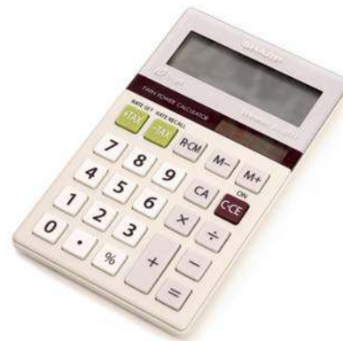
Figure 20.40 The strip of solar cells just above the keys of this calculator convert light to electricity to supply its energy needs. (credit: Evan-Amos, Wikimedia Commons)
