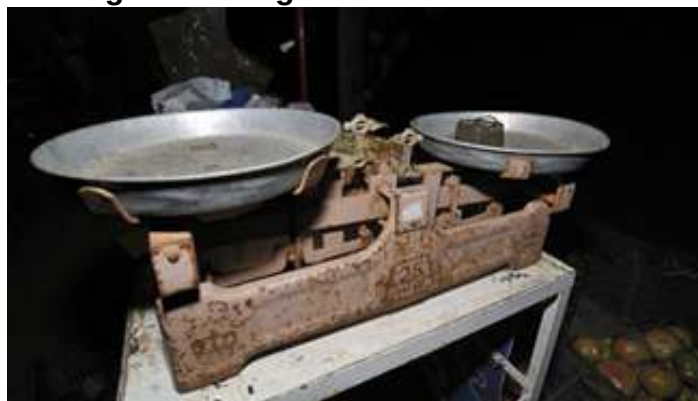
Figure 1.22 A double-pan mechanical balance is used to compare different masses. Usually an object with unknown mass is placed in one pan and objects of known mass are placed in the other pan. When the bar that connects the two pans is horizontal, then the masses in both pans are equal. The “known masses” are typically metal cylinders of standard mass such as 1 gram, 10 grams, and 100 grams. (credit: Serge Melki)
