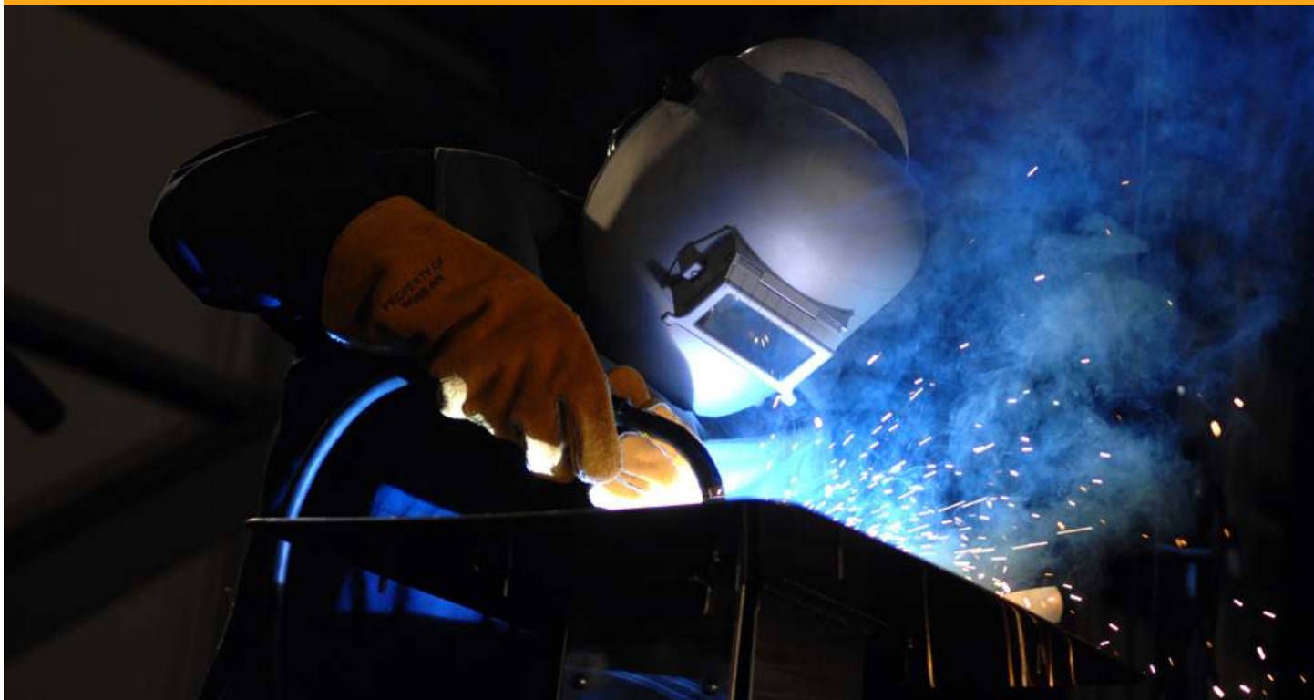
Figure 13.1 The welder's gloves and helmet protect him from the electric arc that transfers enough thermal energy to melt the rod, spray sparks, and burn the retina of an unprotected eye. The thermal energy can be felt on exposed skin a few meters away, and its light can be seen for kilometers. (credit: Kevin S. O'Brien/U.S. Navy)
