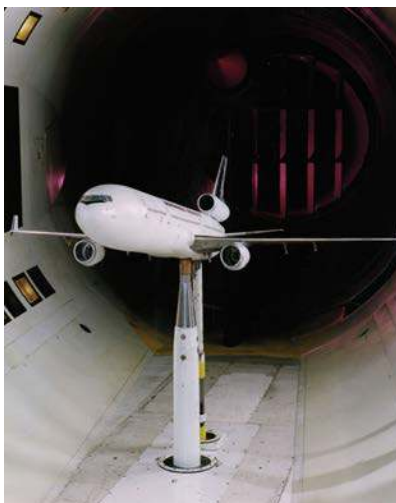
Figure 5.9 NASA researchers test a model plane in a wind tunnel. (credit: NASA/Ames)
