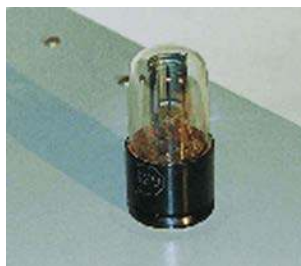
Figure 29.7 The photoelectric effect can be observed by allowing light to fall on the metal plate in this evacuated tube. Electrons ejected by the light are collected on the collector wire and measured as a current. A retarding voltage between the collector wire and plate can then be adjusted so as to determine the energy of the ejected electrons. For example, if it is sufficiently negative, no electrons will reach the wire. (credit: P.P. Urone)
