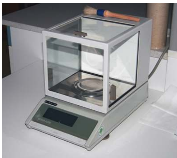
Figure 1.23 Many mechanical balances, such as double-pan balances, have been replaced by digital scales, which can typically measure the mass of an object more precisely. Whereas a mechanical balance may only read the mass of an object to the nearest tenth of a gram, many digital scales can measure the mass of an object up to the nearest thousandth of a gram. (credit: Karel Jakubec)
