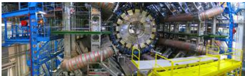
Figure 4.28 The world's largest particle accelerator spans the border between Switzerland and France. Two beams, traveling in opposite directions close to the speed of light, collide in a tube similar to the central tube shown here. External magnets determine the beam's path. Special detectors will analyze particles created in these collisions. Questions as broad as what is the origin of mass and what was matter like the first few seconds of our universe will be explored. This accelerator began preliminary operation in 2008. (credit: Frank Hommes)
