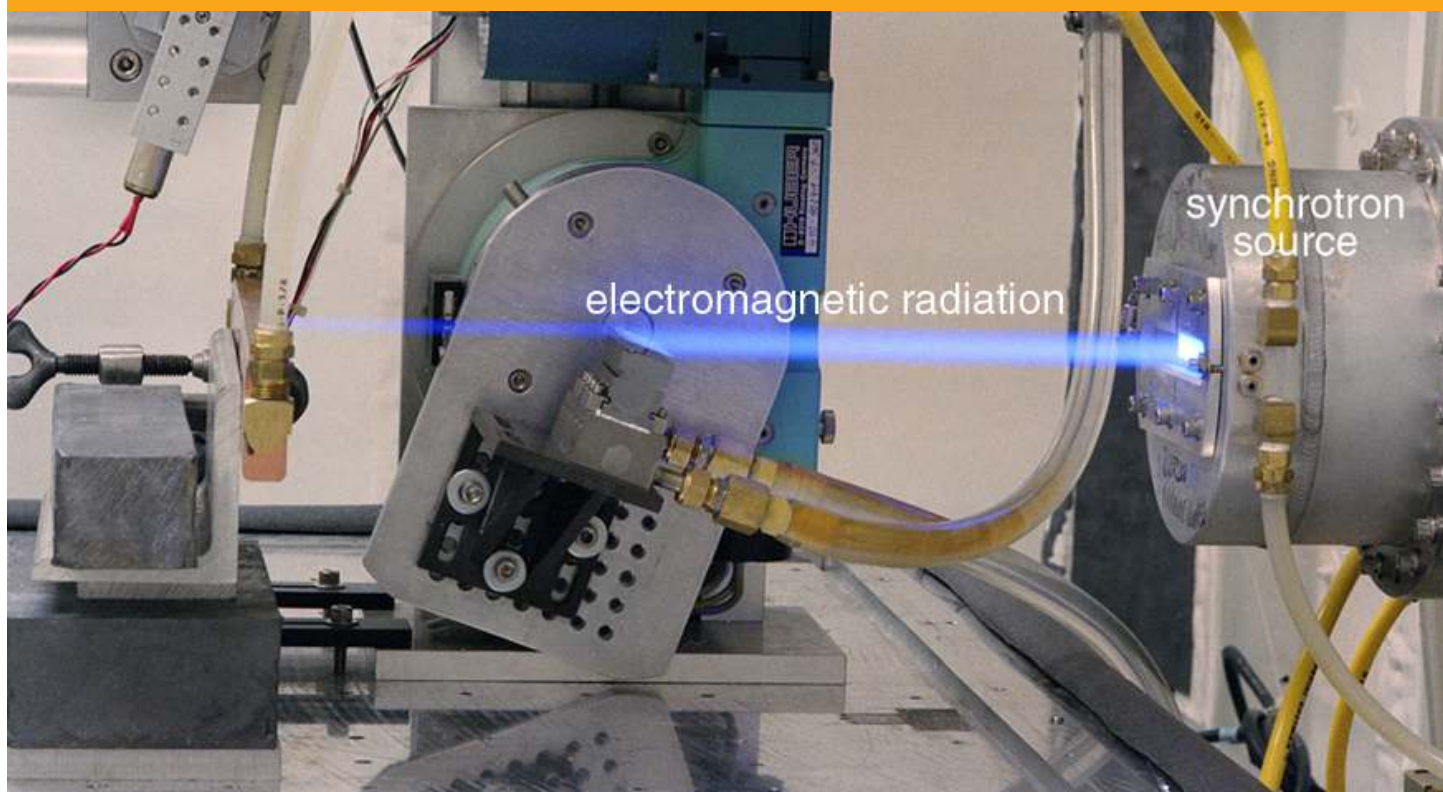
Figure 31.1 The synchrotron source produces electromagnetic radiation, as evident from the visible glow. (credit: United States Department of Energy, via Wikimedia Commons)
