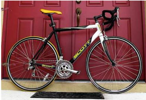
Figure 10.32 The image shows a side view of a racing bicycle. Can you see evidence in the design of the wheels on this racing bicycle that their moment of inertia has been purposely reduced? (credit: Jesús Rodríguez)
