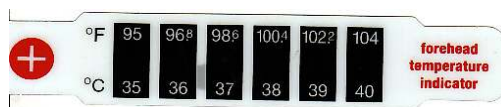
Figure 13.4 Each of the six squares on this plastic (liquid crystal) thermometer contains a film of a different heat-sensitive liquid crystal material. Below 95^{\circ}\text{F} , all six squares are black. When the plastic thermometer is exposed to temperature that increases to 95^{\circ}\text{F} , the first liquid crystal square changes color. When the temperature increases above 96.8^{\circ}\text{F} the second liquid crystal square also changes color, and so forth. (credit: Arkrishna, Wikimedia Commons)
