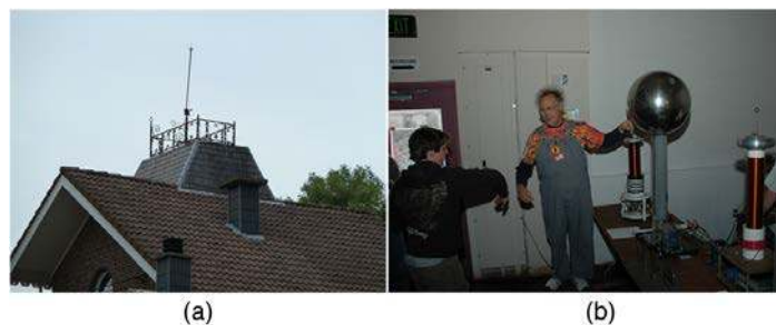
Figure 18.37 (a) A lightning rod is pointed to facilitate the transfer of charge. (credit: Romaine, Wikimedia Commons) (b) This Van de Graaff generator has a smooth surface with a large radius of curvature to prevent the transfer of charge and allow a large voltage to be generated. The mutual repulsion of like charges is evident in the person's hair while touching the metal sphere. (credit: Jon 'ShakataGaNai' Davis/Wikimedia Commons).
