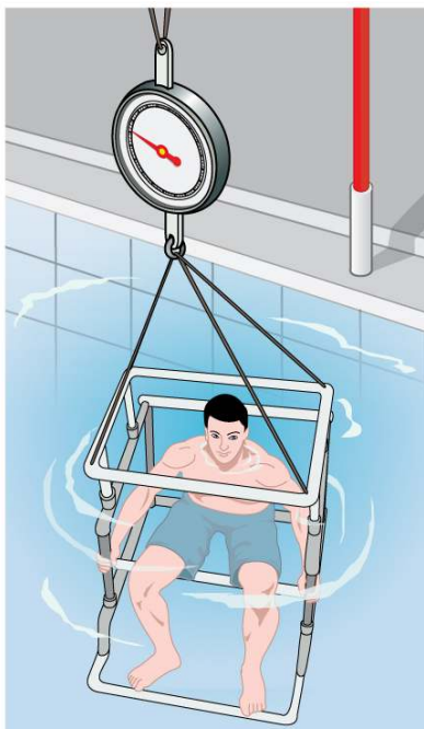
Figure 11.24 Subject in a “fat tank,” where he is weighed while completely submerged as part of a body density determination. The subject must completely empty his lungs and hold a metal weight in order to sink. Corrections are made for the residual air in his lungs (measured separately) and the metal weight. His corrected submerged weight, his weight in air, and pinch tests of strategic fatty areas are used to calculate his percent body fat.
